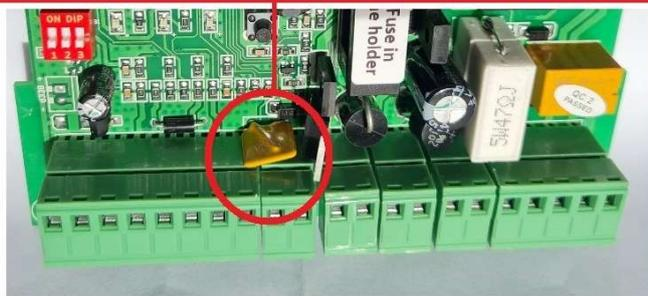
Older PC board - No capacitor fitted.
