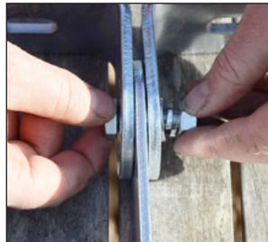
Secure in place with the M10 nut
