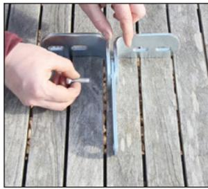
Post pivot bracket in between the two post brackets
